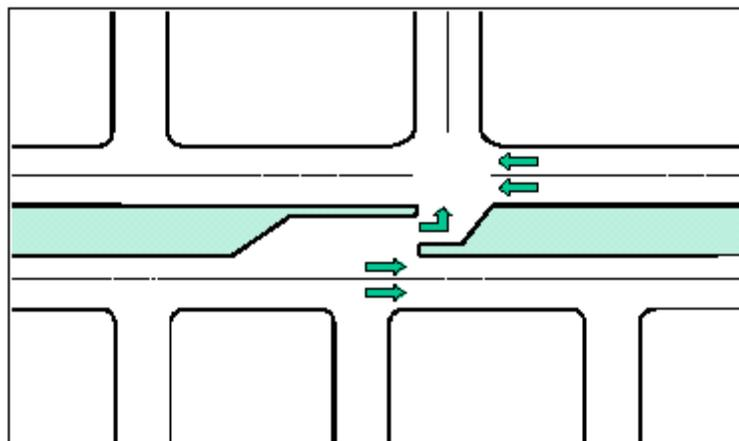
*The directional median break allows for left turns onto the side street. The median prevents vehicles from crossing the arterial and making left turns from side streets onto the arterial.*
