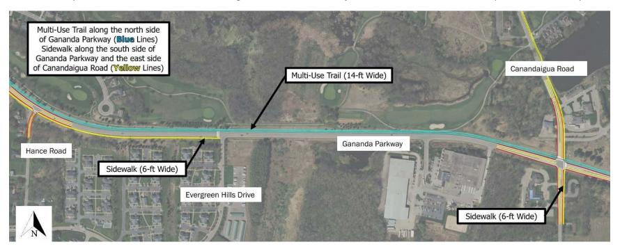
improvements, modifications to the intersection of Canandaigua Road and Gananda Parkway are recommended. Two alternatives are presented as options for the intersection: a 3-phase traffic signal with left turn lanes, and a roundabout.
